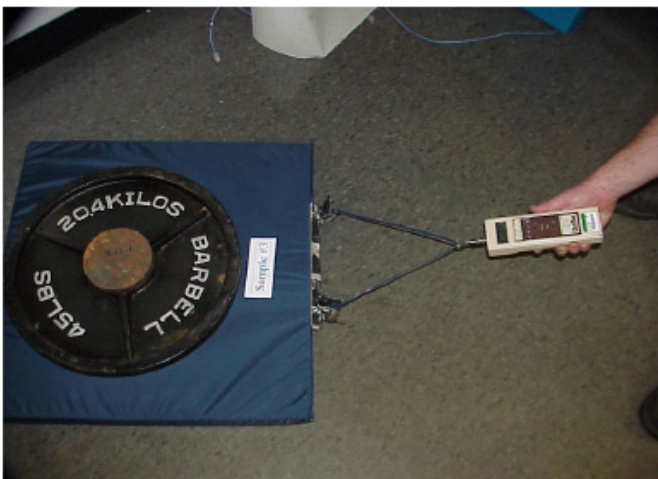
Pull test (representative). Sample No. 3.
