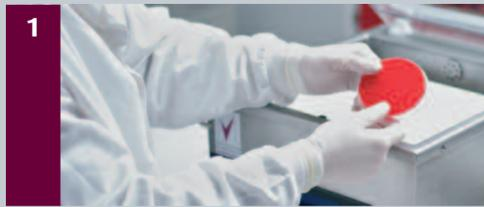
Place your culture media plates, identification strips or samples in the appropriate application bags (use oxygen catalysers with application bags for anaerobic/micro-aerophilic culture for anaerobic atmosphere).
